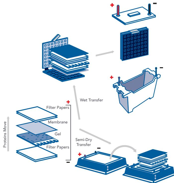
Representative diagrams of the transfer sandwich setup for tank transfer and semi-dry transfer. The membrane is oriented nearest to the positive electrode while the gel is situated towards the negative electrode. The SDS-bound negatively charged proteins will thus migrate out of the gel and onto the membrane.
