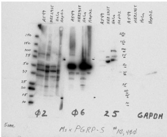
Example of non-specific bands and poor transfer. Target Protein expected at ~25 kDa is not found. Other bands shown are non-specific.
