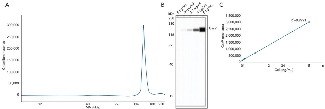
Detection of recombinant Cas9 by Wes, a Simple Western™ instrument. (A) Electropherogram of Cas9 detected by a chemiluminescence readout, (B) lane view of Cas9 detection and (C) linearity analysis of Cas9 detection. Cas9 was detected with the CRISPR-Cas9 Monoclonal Antibody (1013816) (R&D Systems Catalog # MAB10252)
