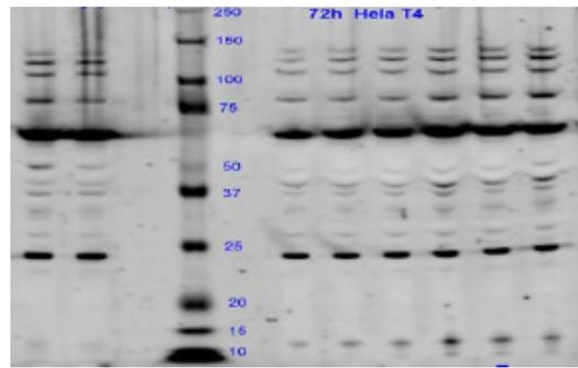
Example of gel run too hot or too high voltage. Results in smiling or misshapen bands. This phenomenon can also occur with poor gel preparation and polymerization.
