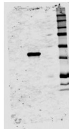
Example of either bacterial contamination or undissolved blocking buffer. Speckled background as a result.
