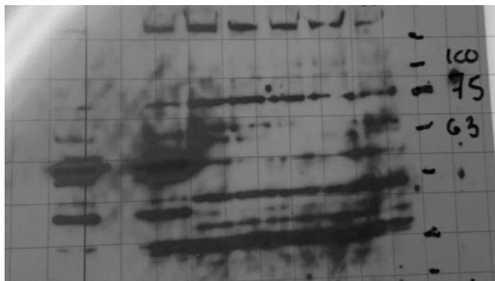
Example of high background and smeared bands. Likely occurred from insufficient blocking or insufficient washing.
