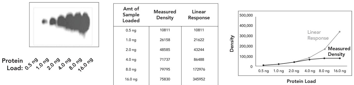
Comparison of the densitometry readings of each sample to the linear response indicates the signal becomes saturated above 4.0 ng. Above 4.0 ng, the band intensity is no longer proportional to total protein abundance: the signal falls outside the linear range of detection. These data determine the optimal total protein load to be 4.0 ng or less for accurate quantification of protein expression.
