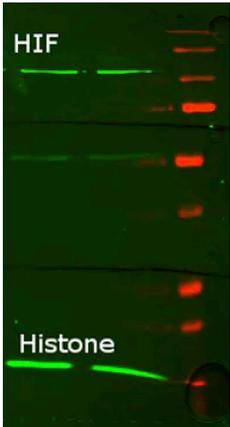
**Example of multiplexing in a fluorescent western.** The blot shows simultaneous probing for two different antibodies, Rabbit Anti-HIF-1 alpha Polyclonal Antibody (Novus Biologicals Catalog # NB100-449) and the loading control Histone, followed by fluorescent dye-conjugated secondary antibody. The protein standard is in the far right lane. Scanned using LI-COR Odyssey system. Image provided by verified customer review from Dr. Lidan Zhao.
