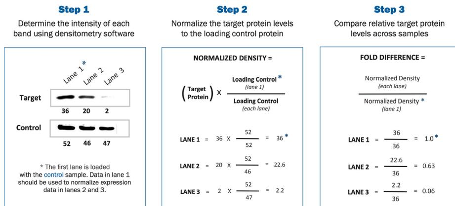
After band intensity is determined by densitometry software, the loading control protein is used to normalize target protein expression. To normalize expression, multiply the density of the target protein in each lane by the ratio of loading control density from the control sample (lane 1) to the loading control density of other lanes. The fold change can then be calculated by dividing the normalized expression from each lane by the normalized expression of the control sample in lane 1.
