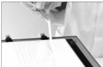
Fig 3.5. Applying an electrode strip near the anode.
