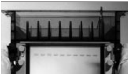
Fig 2.8. Locking the upper buffer chamber in place.
