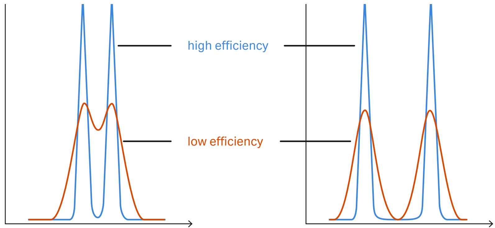
Fig 1.12. Resolution depends both on the selectivity and the efficiency of the resin.
