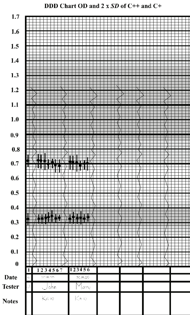
Fig. 19. DDD chart of OD data. Tests done on three days: the 9th, 20th, and 30th of a month. Two operators conducted the tests.
